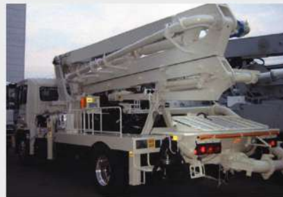
Concrete Pump Truck
